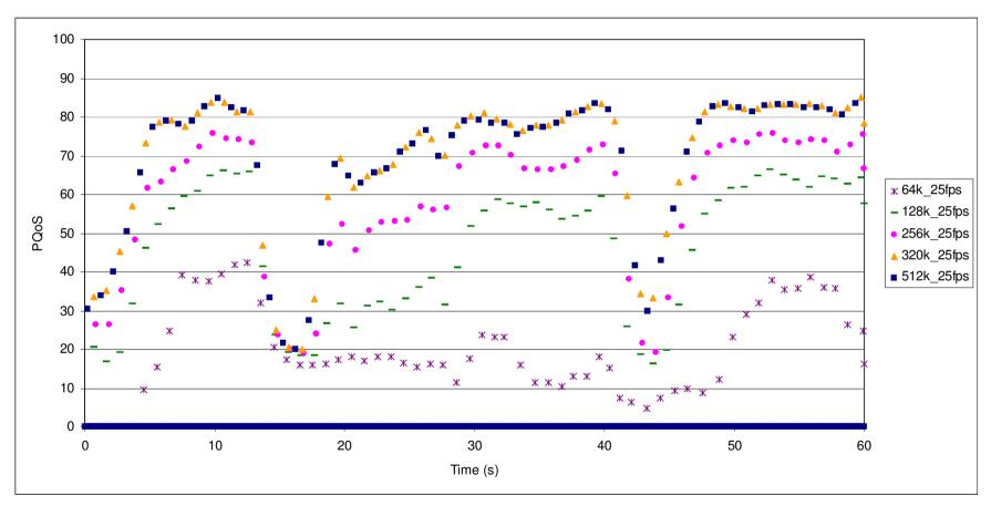
Continuous measurements, for different encoding data rates 64 .. 512 kbit/s Clear impact on PQoS; PQoS average is well correlated to subjective tests results
