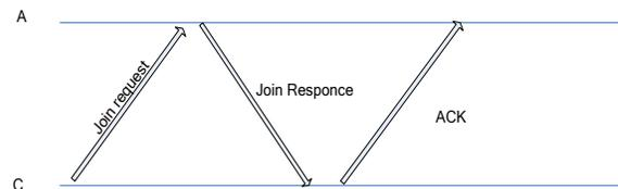
Fig.2 The procedures of a three-way handshake.
