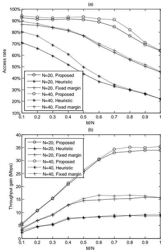
Figure 2. D2D access rate and throughput gain
