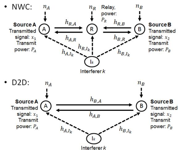
Figure 3: Signal models for NWC and D2D transmissions.
