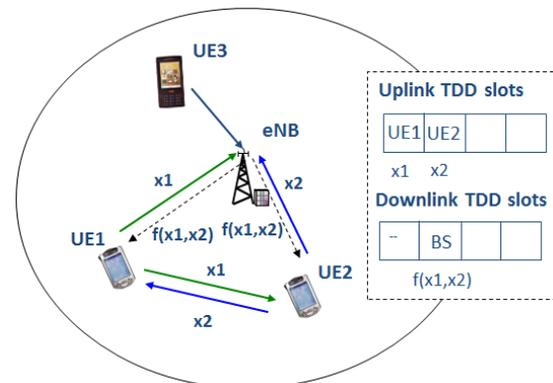
Figure 1: D2D and NWC technologies integrated in a cellular network.
