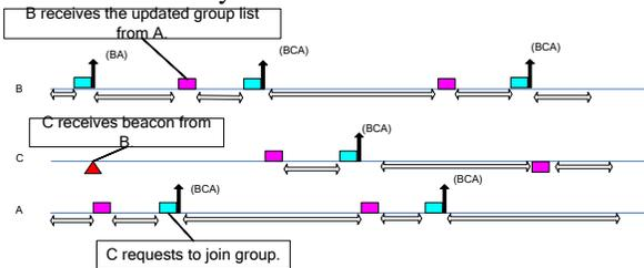
Fig. 3 The procedures of a device joining a group.
