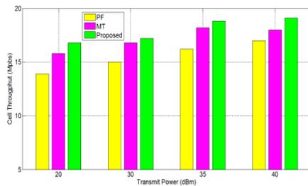
Figure 3: Cell center Throughput vs. transmit power
