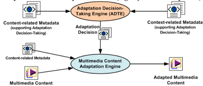
Figure 1. High-level Architecture of Adaptation Decision-Taking and Multimedia Content Adaptation.
