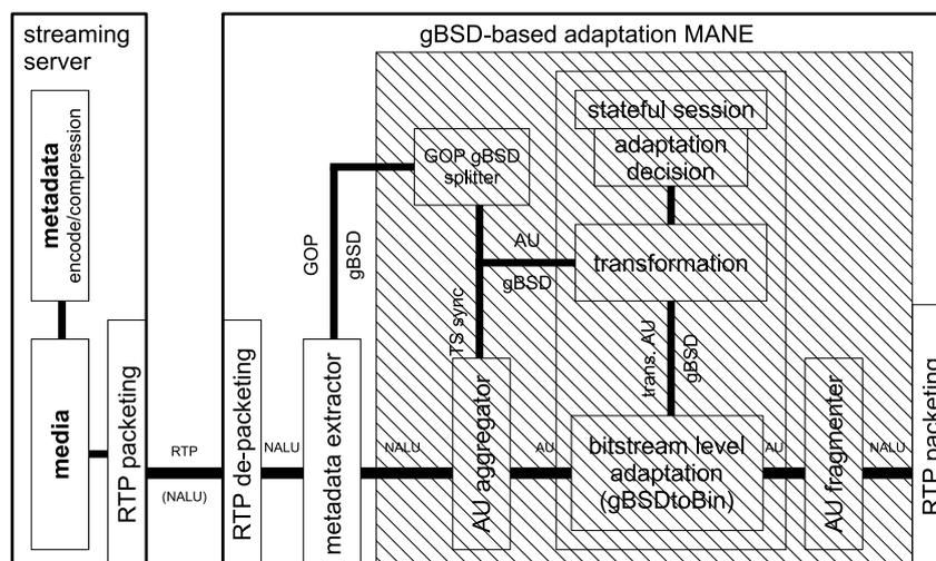
Fig. 6. gBSD single-stream solution.
