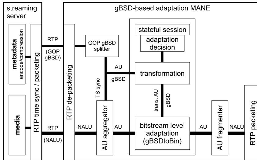
Fig. 5. gBSD two-stream solution.
