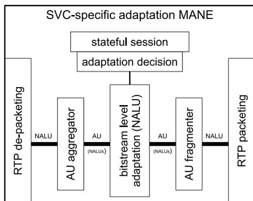
Fig. 3. SVC-specific adaptation based on NAL units.
