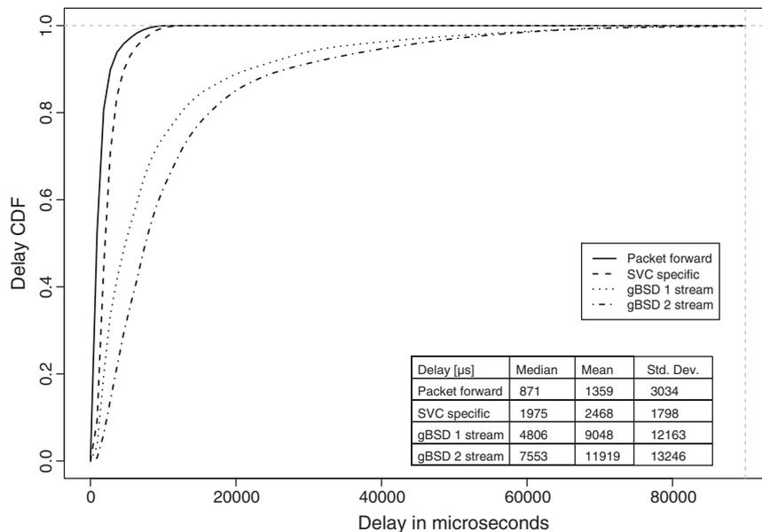
Fig. 12. Delay distribution function for sequence *harbour mgs2 GOP32*.
