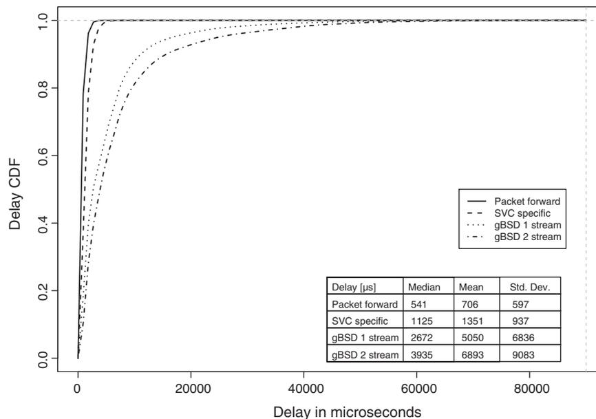
Fig. 10. Delay distribution function for sequence *foreman mgs* GOP32.
