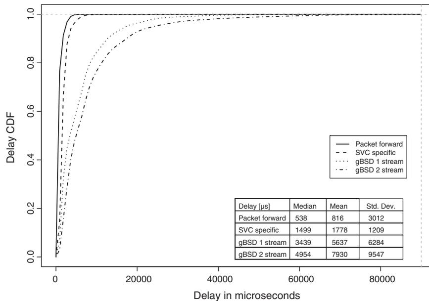
Fig. 11. Delay distribution function for sequence *city mgs2 GOP32*.
