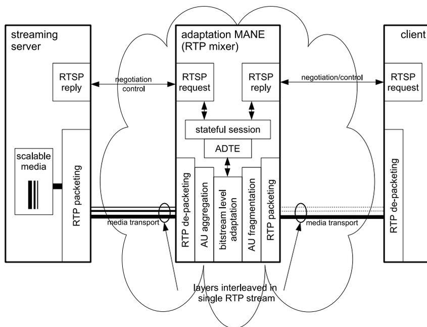
Fig. 2. Adaptation-enabled MANE based on RTSP/RTP.
