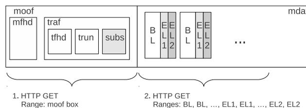
Fig. 2. Priority streaming of a single fragment based on the *subs* box
