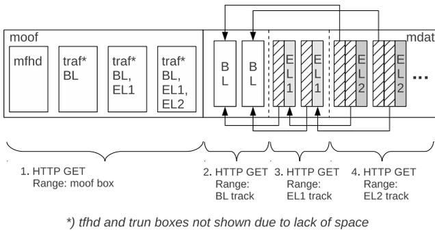
Fig. 3. Priority streaming of a single fragment using multiple tracks
