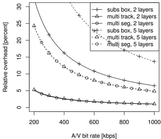
Fig. 5. Overhead analysis for low bit rate content
