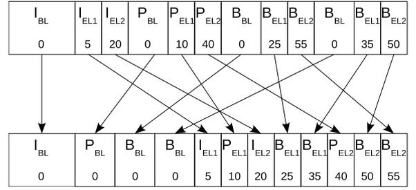
Figure 6: PRID-based NAL unit reordering
