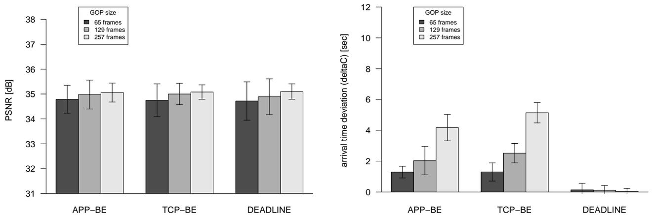
**Figure 10: Underprovisioned network:  $BW = 1536$  kbps. PSNR and arrival time deviation on the client ( $\delta C$ ) for the different algorithms and GOP sizes at 200 ms RTT.**
