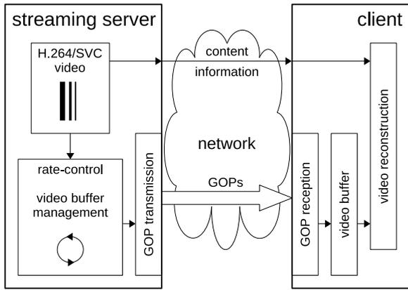
Figure 3: Server-side adaptive streaming system
