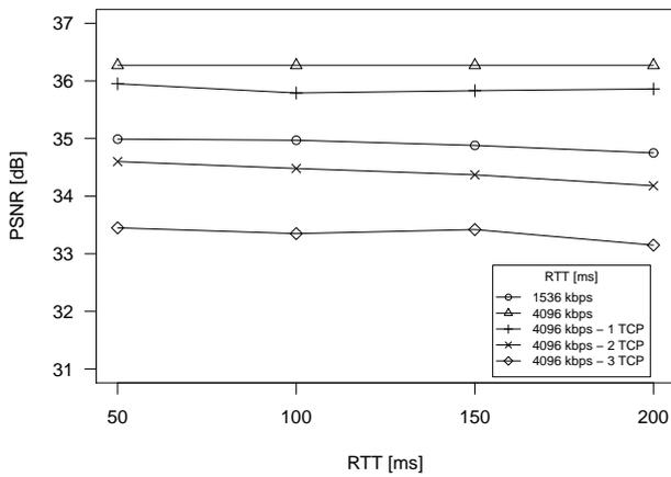
Figure 15: Average PSNR for TCP-BE with GOP size 65 with respect to the RTT.
