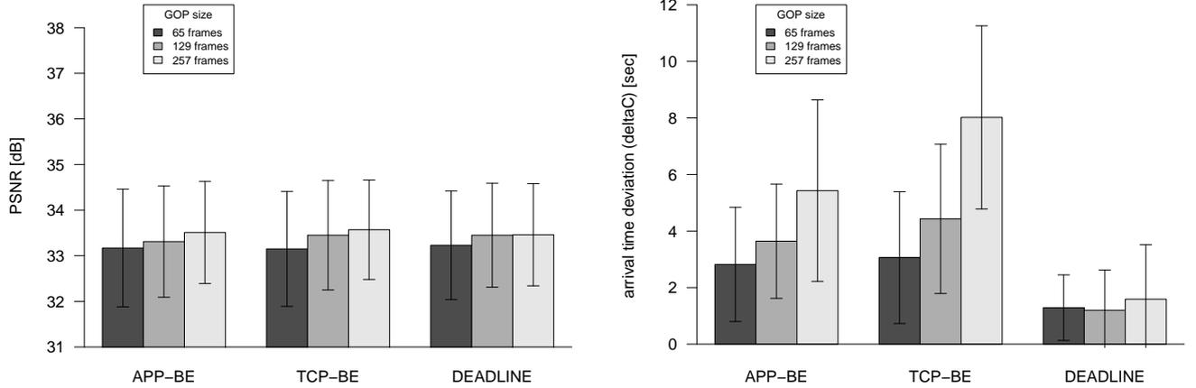
**Figure 13: Congested network:  $BW = 4096$  kbps and three concurrent TCP streams. PSNR and arrival time deviation on the client ( $\delta C$ ) for the different algorithms and GOP sizes at 200 ms RTT.**
