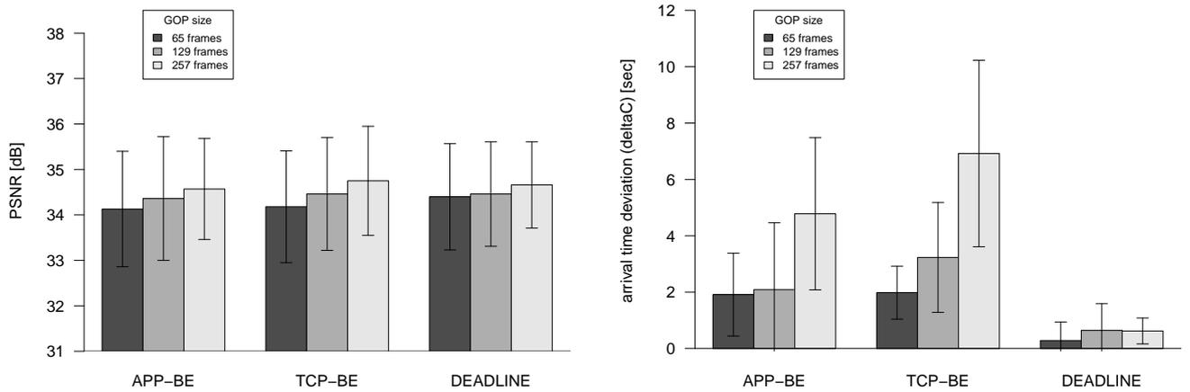
Figure 12: Congested network:  $BW = 4096 \text{ kbps}$  and two concurrent TCP streams. PSNR and arrival time deviation on the client ( $\text{delta}C$ ) for the different algorithms and GOP sizes at 200 ms RTT.
