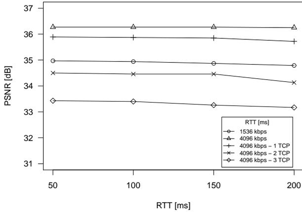
Figure 14: Average PSNR for APP-BE with GOP size 65 with respect to the RTT.
