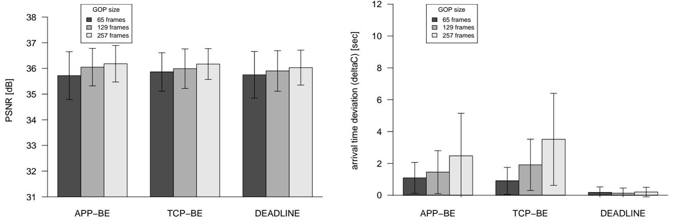
Figure 11: Congested network:  $BW = 4096 \text{ kbps}$  and one concurrent TCP stream. PSNR and arrival time deviation on the client ( $\text{delta}C$ ) for the different algorithms and GOP sizes at 200 ms RTT.
