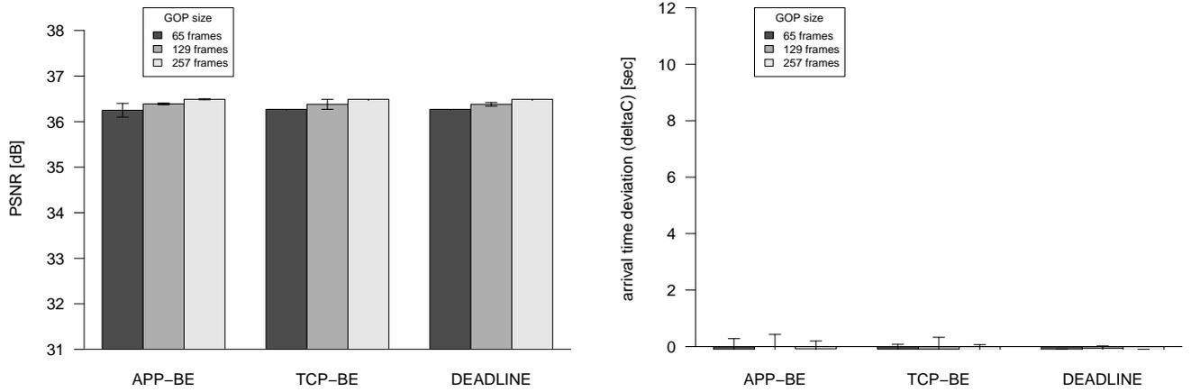
**Figure 9: Overprovisioned network:  $BW = 4096$  kbps. PSNR and arrival time deviation on the client ( $\delta C$ ) for the different algorithms and GOP sizes at 200 ms RTT.**
