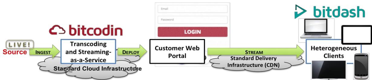
Figure 1: High-Level System Architecture for Live Transcoding and Streaming-as-a-Service.
