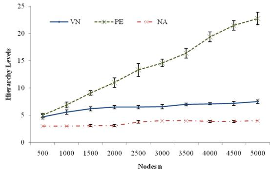
Figure 3. Hierarchy depth on random dense ON; different numbers of nodes.
