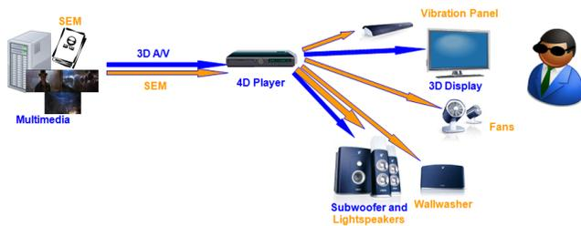
**Figure 1. Overview of Enriched 3D Multimedia Playback.** filters of the commercial Stereoscopic Player [8]. The Stereoscopic Player provides a number of different 3D modes such as side-by-side, interleaved, anaglyph, or NVIDIA 3D Vision/AMD HD3D.
