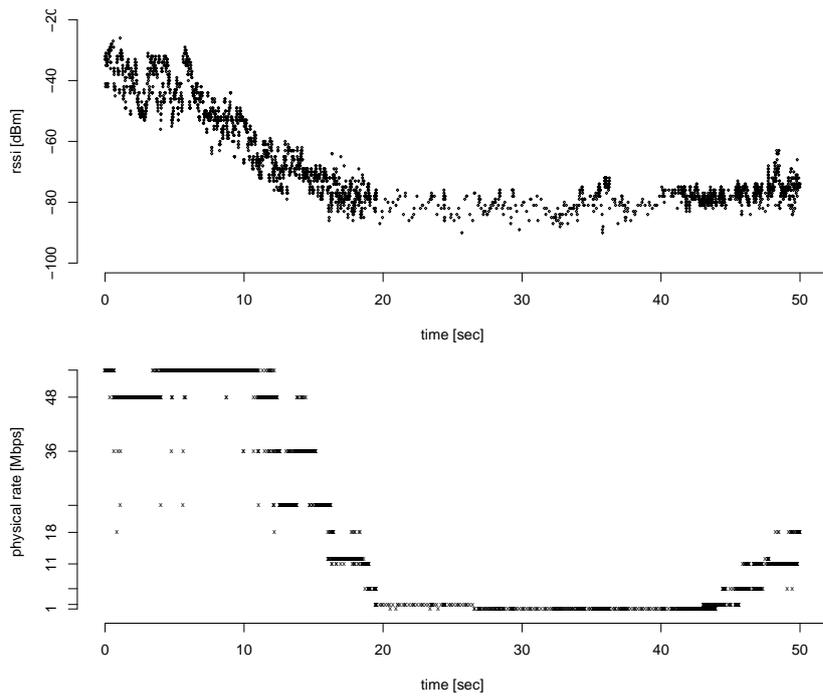
Fig. 3 Signal strength and physical rate – Dlink AP
