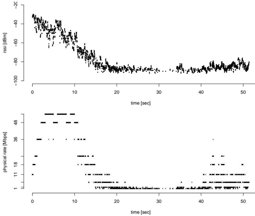
**Fig. 2** Signal strength and physical rate – Linksys AP
