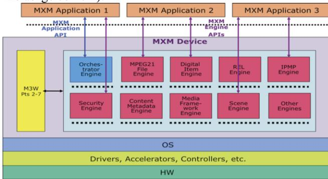
Figure 1. The MXM Architecture.
