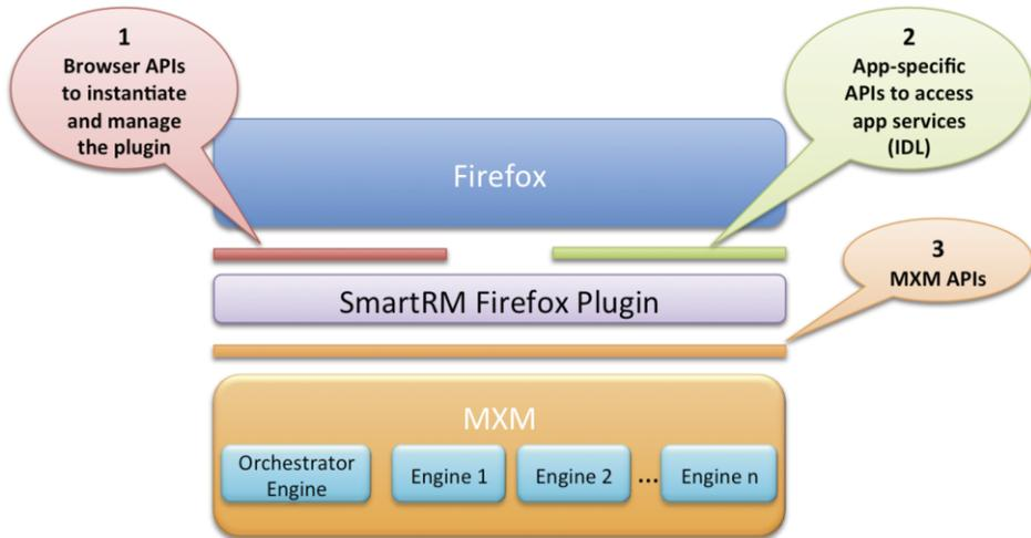
Figure 6. High-level architecture of the SmartRM MXM-based Firefox plug-in.
