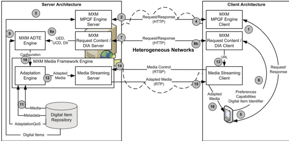
Figure 4. MXM-based Architecture for a Fully Interoperable Streaming Framework of Media Resources in Heterogeneous Environments.
