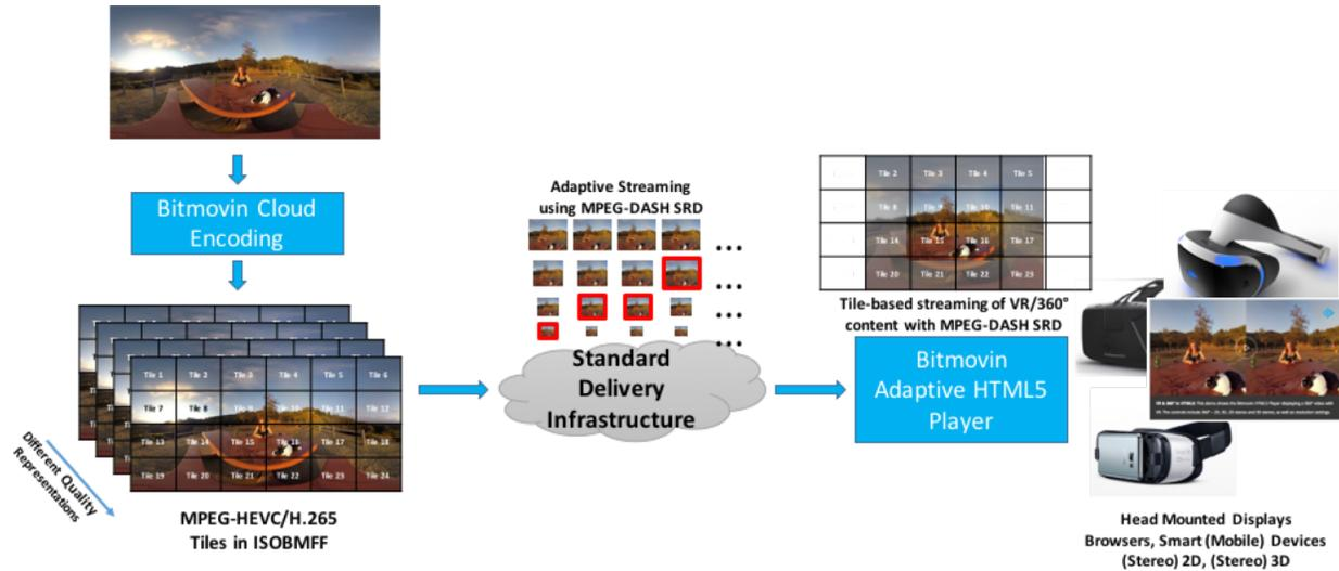
FIGURE 2. EXAMPLE WORKFLOW OF ADAPTIVE STREAMING OF IMMERSIVE MEDIA SERVICES.
