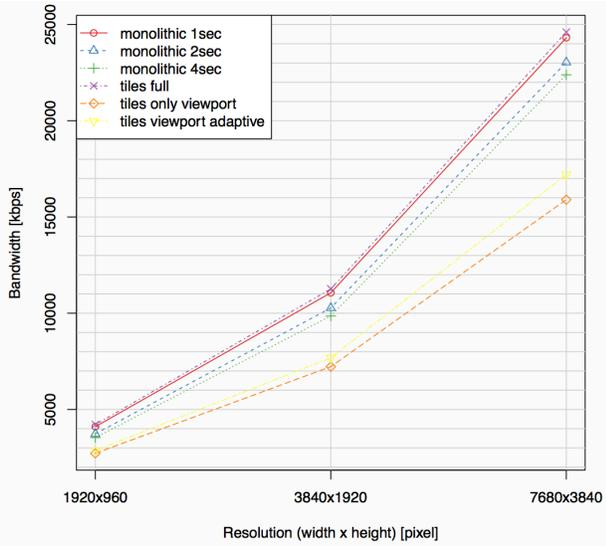
FIGURE 5. BANDWIDTH REQUIREMENTS, 3X2 TILES.
