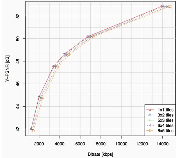
FIGURE 4. TILE OVERHEAD FOR RESOLUTION 7680X3840.
