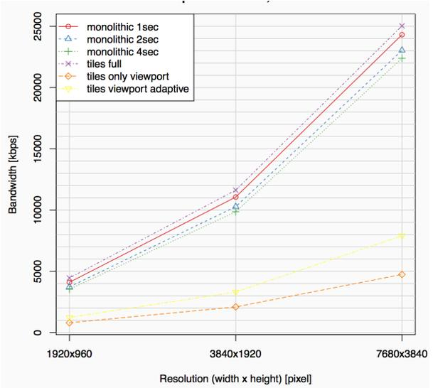
FIGURE 6. BANDWIDTH REQUIREMENTS, 6X4 TILES.
