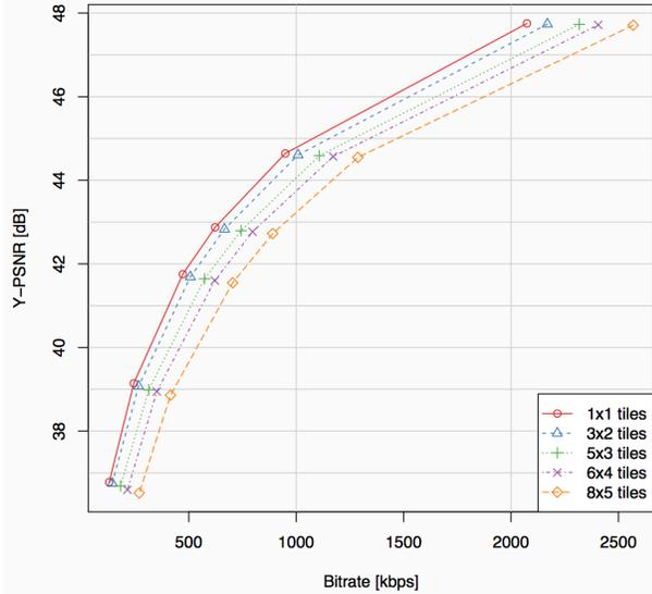
FIGURE 3. TILE OVERHEAD FOR RESOLUTION 1920X960.
