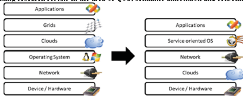
Figure 3: layer model without (left) and with (right) Service oriented Operating Systems
