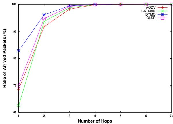
Fig. 5. Cumulative distribution function of the hop count
