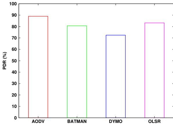
Fig. 2. Average packet delivery ratio of the four routing protocols
