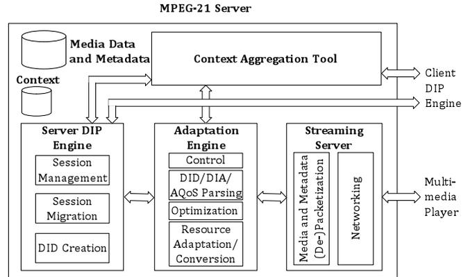
Figure 2. DANAE MPEG-21 Server Architecture.
