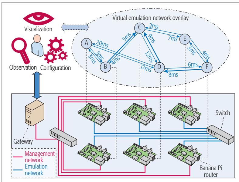
Figure 1. An overview of the testbed architecture. The testbed consists of two dedicated physical networks. The management network (red lines) is used to set up and control the testbed nodes, while the emulation network (blue lines) realizes the virtual overlay network. The gateway is used as a control server, and enables users to configure, observe, and visualize emulation tasks.
