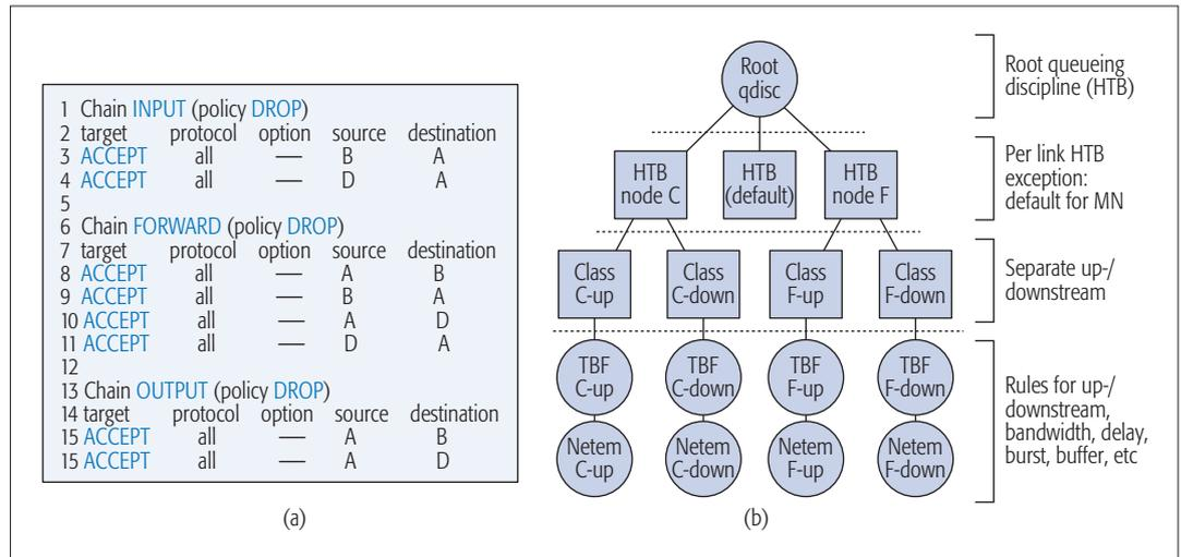
Figure 2. The left side sketches the configuration of the Linux iptables by the example of node A (Fig. 1). The right side illustrates the Linux traffic control classification for packet scheduling by the example of node E.
