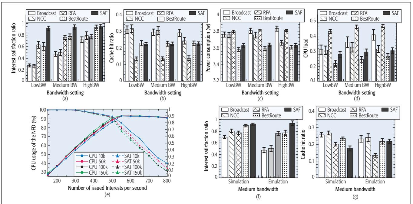
Figure 4. The figure depicts the findings of the conducted experiments. Subfigures 4a–d illustrate the results obtained from the testbed. Subfigures 4f and 4g compare the results obtained by emulations and simulations for the setting “MediumBW” also. Subfigure 4e indicates the packet processing capabilities of a BPI-R1 with respect to varying cache sizes (10,000–150,000 entries).
