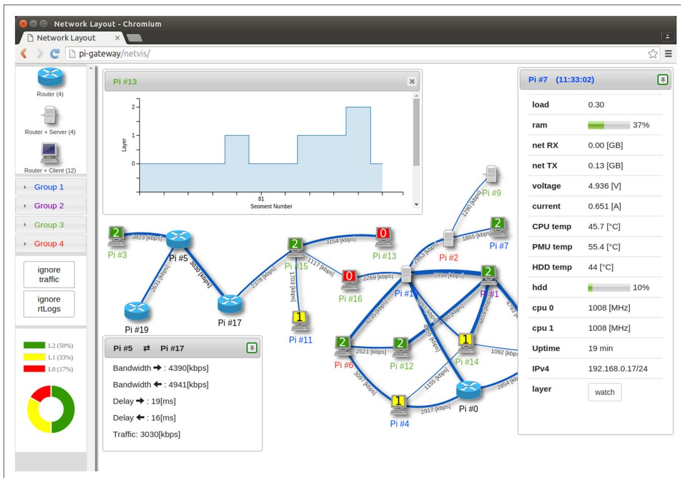
Figure 3. Snapshot of the web interface that can be used to monitor ongoing emulations in near real time.
