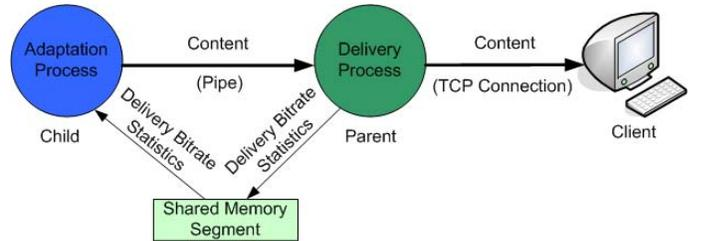
Fig. 1. Interprocess communication between delivery module and adaptation engine.
