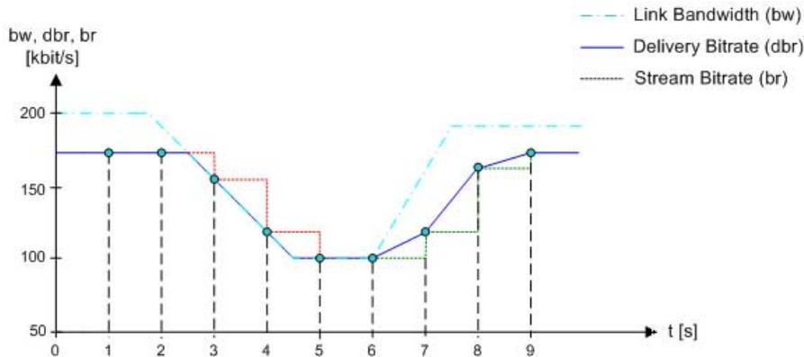
Fig. 2. Handling Bandwidth Fluctuations
