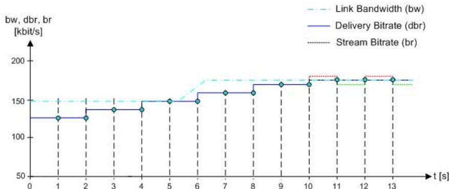
Fig. 3. Available Bandwidth Detection
