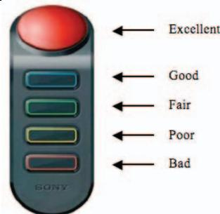
Figure 2. Voting device and mapping to voting scale.
