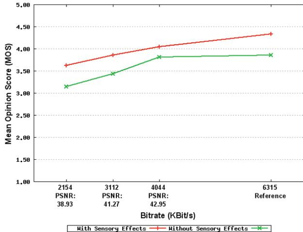
Figure 9. MOS vs. PSNR/bit-rate for Babylon A.D.
