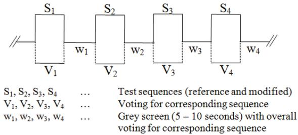
Figure 1. Testing method.
