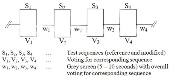
Figure 1. Testing method.
