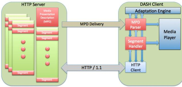
**Figure 1: MPEG-DASH-based System Architecture.**
