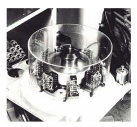
Original logic units of the computer (left to right: first, two combined gates, second, two flip-flops)
